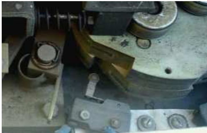
Earlier design employing hinged roller microswitches – Ratchet Activated
