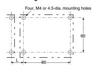
Note: If more than one Power Supply is installed in a row, keep a distance of 20 mm min. (L = 20 mm min.) between each adjacent Power Supply.
