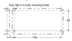
Note: If more than one Power Supply is installed in a row, keep a distance of 20 mm min. (L = 20 mm min.) between each adjacent Power Supply.
