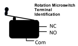
When Using TCB 6.x to replace previous versions, move wire from NC to NO
