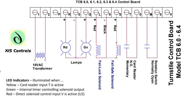
**Reconfigure** – Remove chips U4 & U3. Rotate 6 pin chip so index dot/notch is down and place in socker U2
